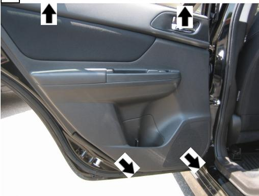
Pull out on bottom of door panel, then lift up to release panel from door. Verify that no clips remain in the metal door. If so, remove them and reinstall them to door panel.
