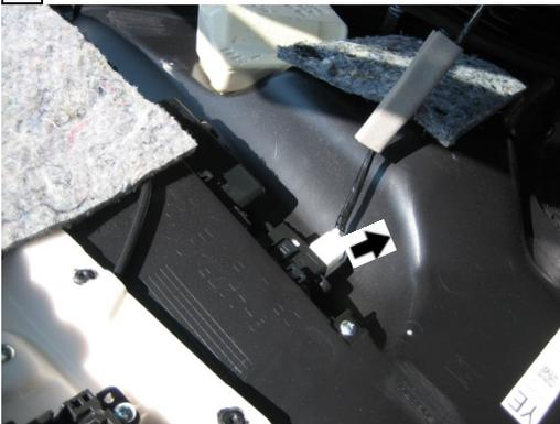
On back side of door panel, unclip wire harness and remove. Carefully place door panel aside.
