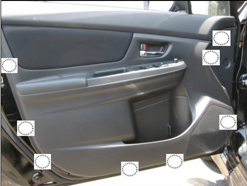
Starting from bottom corner, pry panel from door to release clips (8)
