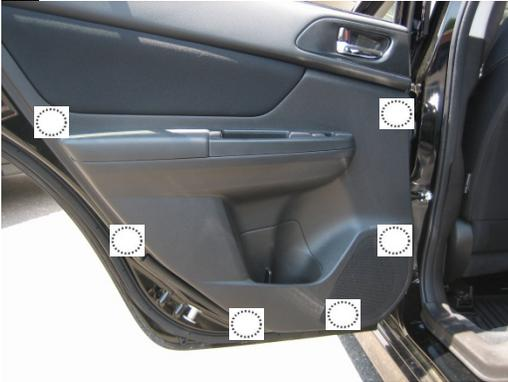
Starting from bottom rear corner, pry panel from door to release clips (6).
